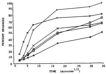
\*M/G=1.34, Ca-alginate \*M/G=1.34, Cu-alginate \$\Delta M/G=1.34, Cr-alginate +M/G=1.65, Ca-alginate \$\Delta M/G=1.65, Cu-alginate \$\Delta M/G=1.65, Cr-alginate
